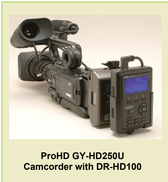
Fig. 8. The DTE (Direct-to-Edit) ProHD hard disk recorder can be attached on top of the camcorder or on the back side of the battery, recording up to 6 hours of live compressed material direct to disk at. The DR-HD100 can be connected via 1394 to a laptop or to a workstation with direct access to the HD material for editing, without the need to transfer to the local disk array before editing. Thus the name “Direct-to-Edit” or DTE. NOTE: DTE and Direct-to-Edit are trademarks of Focus Enhancements Inc.
